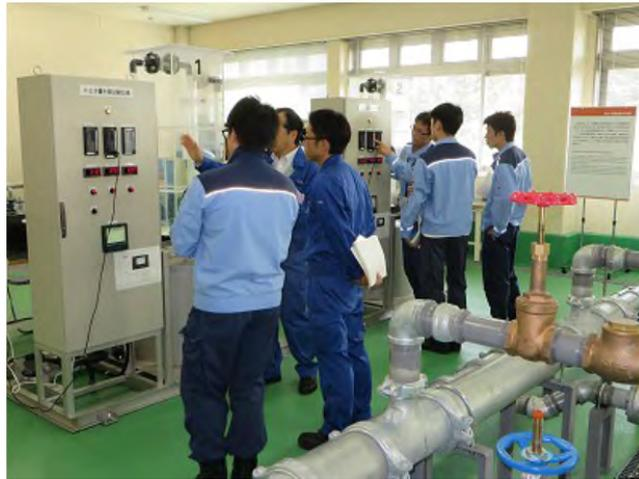
**Figure 16. Water level and flow rate control test equipment**
