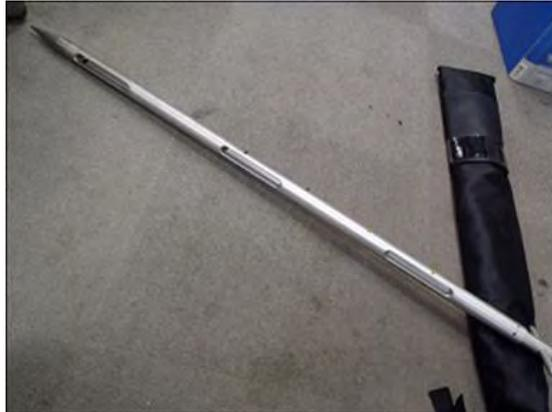
**Figure 4. Zone sampler**
