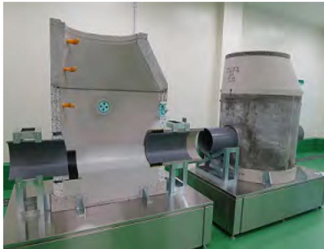
**Figure 5. Cut-model; Manhole earthquake disaster countermeasure Equipment**
