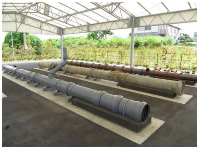
**Figure 13. In-pipeline television camera investigation model**
